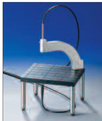
Transmittance maybe measured with a simple stage modification
